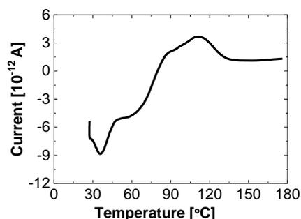
Figure 1: The open-circuit thermally stimulated depolarization current on PLA.
