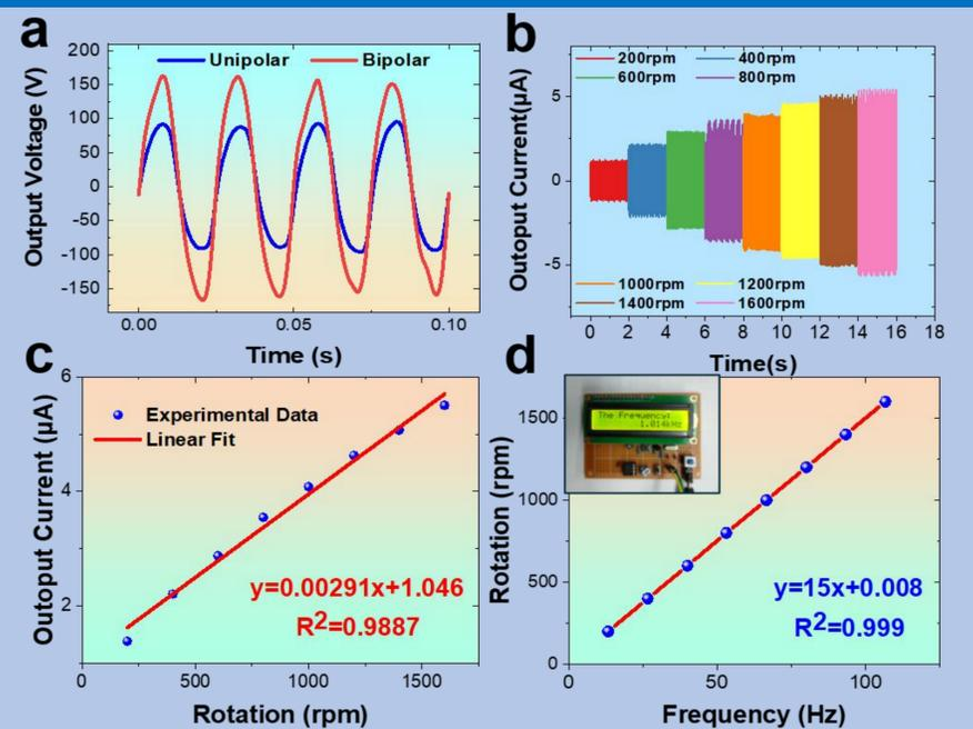
**Figure 2:** Experimental measurement results of the ETBB (a)Comparison of unipolar and bipolar output voltage at 600 rpm (b) Comparison of output current at different rotating speed (c) The relationship between bearing output current and speed based on linear fitting of experimental data (d) Derive the relationship between output current and frequency based on experimental data.
