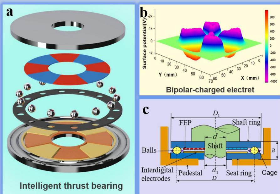
**Figure 1:** : Structural design of the ITBB based on the free-standing mode (a)Structural explosion diagram of the ITBB(b) Measured 3D potential distribution of the ITBB: Blue color depicts the negatively charged area and red color depicts the positively charged area. (c) Installation diagram of the ITBB with the rotor shaft and the bearing seat hole.
