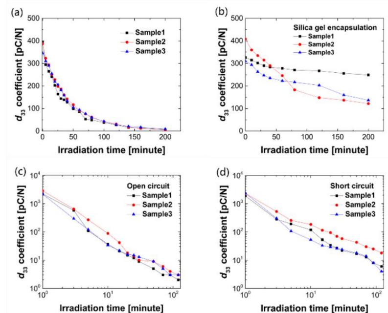
**Figure 1: Decay curves: (a) IXPP films with direct soft X-ray irradiation. (b) IXPP films encapsulated with silica gel. (c) Open-circuited FEP films. (d) Short-circuited FEP films.**
