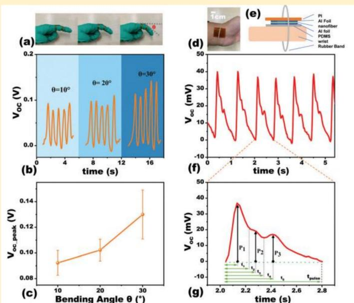
Fig.7 Application of the nanofiber membrane<sub>15:0.1</sub>
