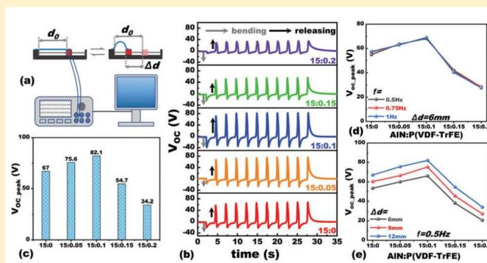
Fig.4 The transverse piezoelectric property.
