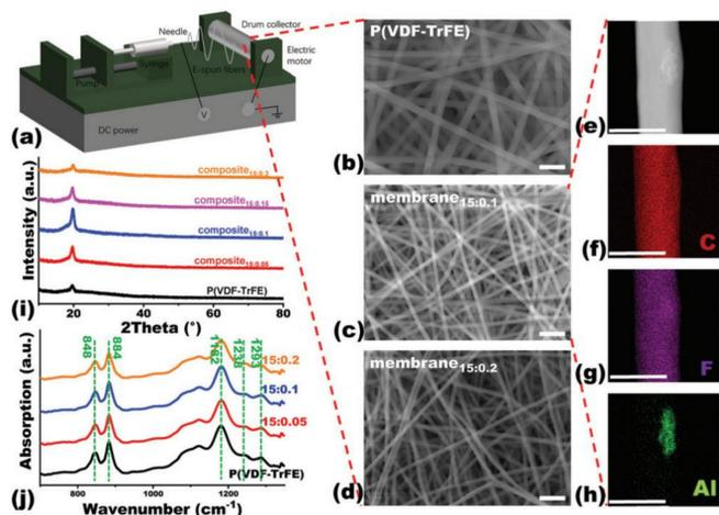
Fig.1 Electrospinning of AlN doped P(VDF-TrFE) nanofibers.
