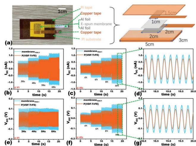
Fig.2 Electrical responses of both the AlN-doped nanofiber membrane<sub>15:0.1</sub> and the neat one.
