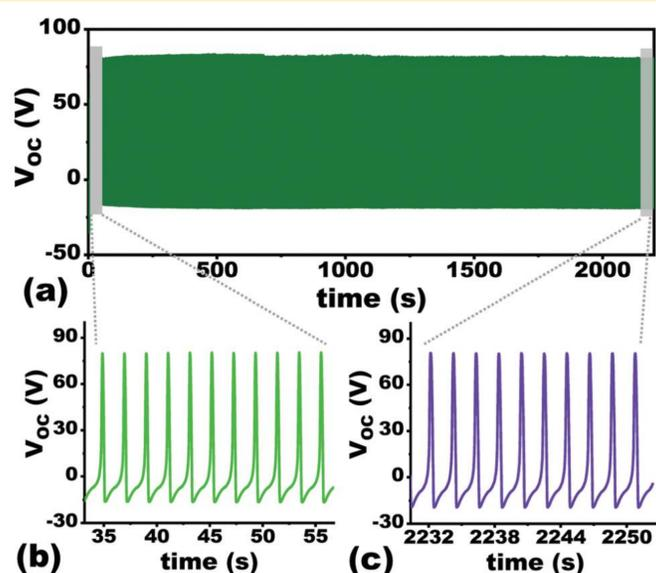
Fig.5 Endurance of the open-circuit voltage response. As for endurance, the output voltage stays stable during 1100 cycles.
