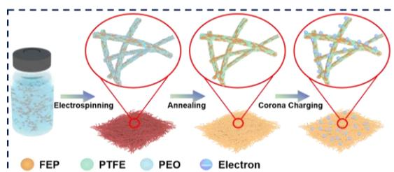
Figure 1. The fabrication method of PFM.
