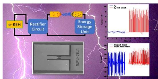
Figure 1: The graphical abstract. The schematic design of the system, SEM image of MEMS needle plasma switch and its voltage and current performance enhancement.
