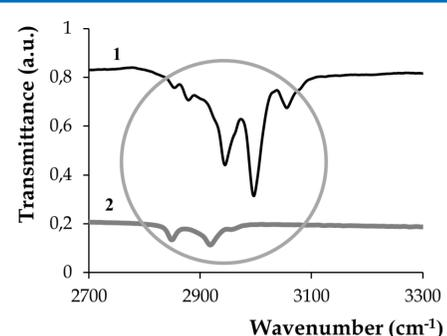
Fig. 4. IR transmittance spectra of films of the initial PLA 40 μm (curve 1) and the ATR spectra of the initial PLA 226 μm (curve 2) in the wavenumber range: a) from 1300 cm<sup>-1</sup> to 1800 cm<sup>-1</sup>; b) from 2700 cm<sup>-1</sup> to 3300 cm<sup>-1</sup>
