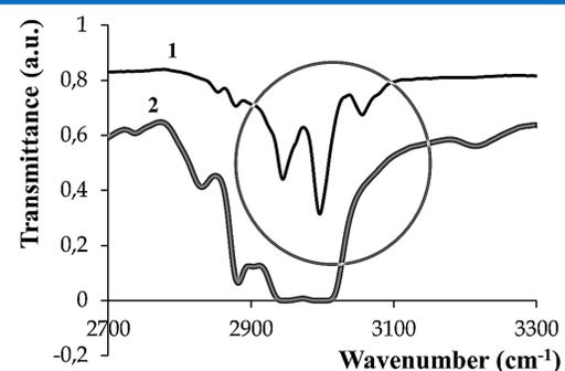
Fig. 3. IR transmission spectra of films of the original PLA with a thickness of 40 μm (curve 1) and 226 μm (curve 2) in the range of wavenumbers: a) from 1300 cm<sup>-1</sup> to 1800 cm<sup>-1</sup>; b) from 2700 cm<sup>-1</sup> to 3300 cm<sup>-1</sup>
