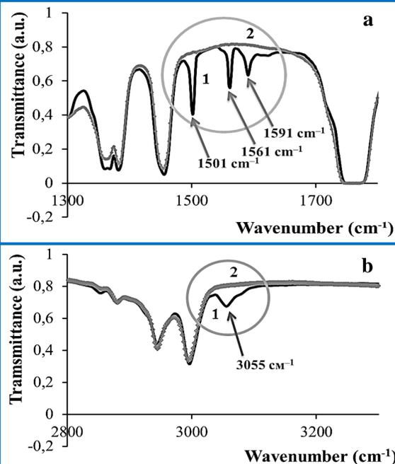
Fig. 2. The IR transmission spectra of the initial PLA (curve 1) and the PLA composite with the hydrophilic filler barium titanate (BaTiO<sub>3</sub>) (curve 2) in the wavenumber range: a) from 1300 cm<sup>-1</sup> to 1800 cm<sup>-1</sup>; b) from 2800 cm<sup>-1</sup> to 3300 cm<sup>-1</sup>
