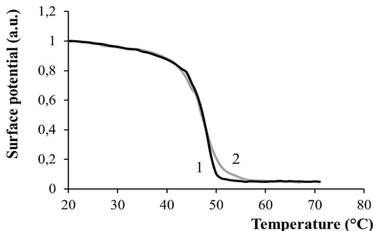
Fig. 1. TSRSP curves of initial PLA at the same heating rate, electreted in the field of negative (curve 1) and positive (curve 2) corona discharge
